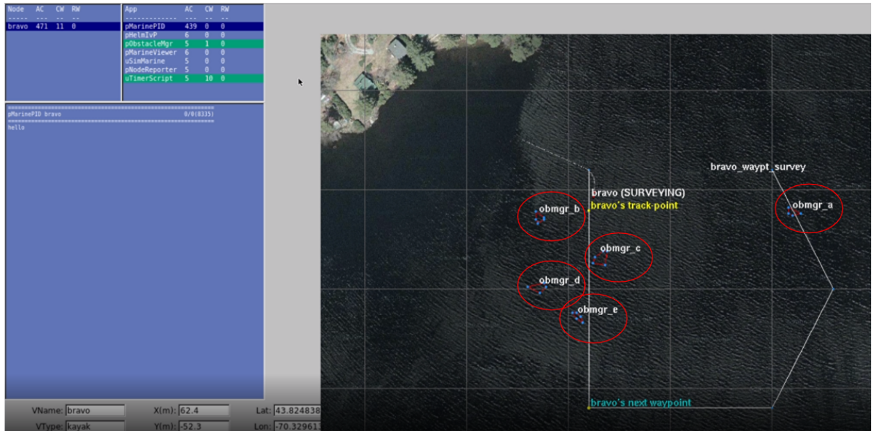
Figure 20. The user interface showing pObstacleManager from our obstacle detection simulation with detected objects circled in red. The simulation shows that the boat is able to detect and avoid obstacles.
